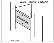
Locate the top of the wood wall framing at 47" from cooktop (see illustration at right). Once wall surface is finished, carefully trace a center line over installation location, then trace a level line at 45" from cooktop. Center and level the hood mounting bracket, secure it to wall framing with 3 no. 8 x 1½" flat head
