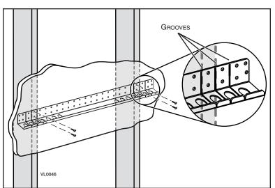
**6** LIFT UNIT AND ENGAGE EACH GROMMET IN THE WALL BRACKET BOTTOM EDGE HOLES. SLIDE A WASHER AND SECURE WITH A CAP NUT (INCLUDED) ON THE BOLT OF EACH ANGLE BRACKET ASSEMBLY TO ENSURE THE UNIT IS KEPT IN PLACE.
