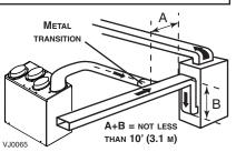
B. FRESH AIR TO BUILDING DUCT AND EXHAUST AIR FROM BUILDING DUCTS
