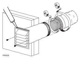
tape. Pull the insulation over the joint. Pull the vapor barrier over the insulation and over the joint. Apply gently duct tape to the joint making an airtight seal. See above.
